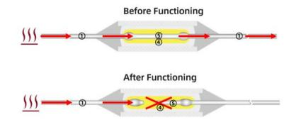
Heat is transferred from the left Lead Wire① to the Fusible Alloy⑤. When the temperature reaches Fusing Temp. fusible alloy⑤ disconnects.
