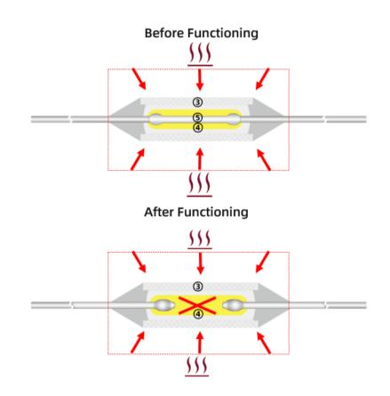
Heat is transferred from the case 3 to the Fusible Alloy 5. When the temperature reaches Fusing Temp. fusible alloy 5 disconnects.
