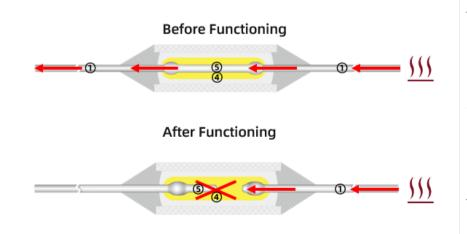
Heat is transferred from the right Lead Wire① to the Fusible Alloy⑤. When the temperature reaches Fusing Temp. fusible alloy⑤ disconnects.
