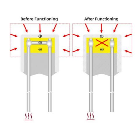
Heat is transferred from the case③ to the Fusible Alloy⑤.
